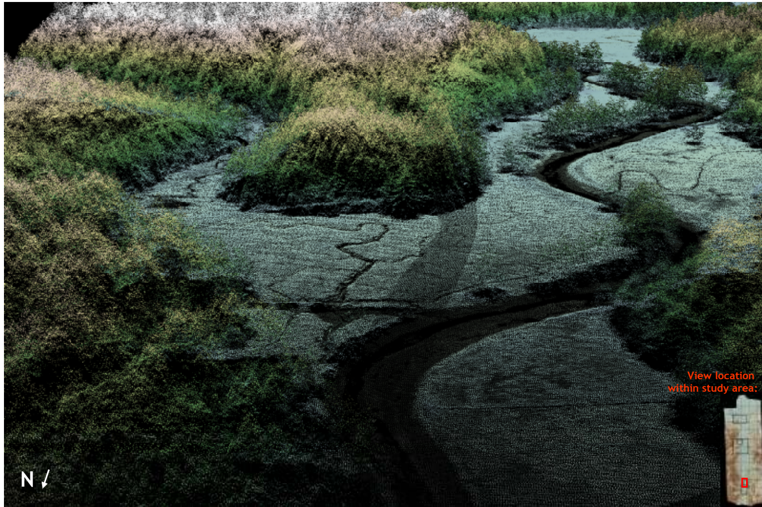
View 4: All laser returns shown as point cloud with intensity
