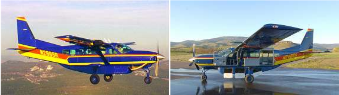
Figure 2. The Cessna Caravan 208 - A removable composite cargo pod provides housing for GPS equipment and the LiDAR system and other remote sensing sensors.
