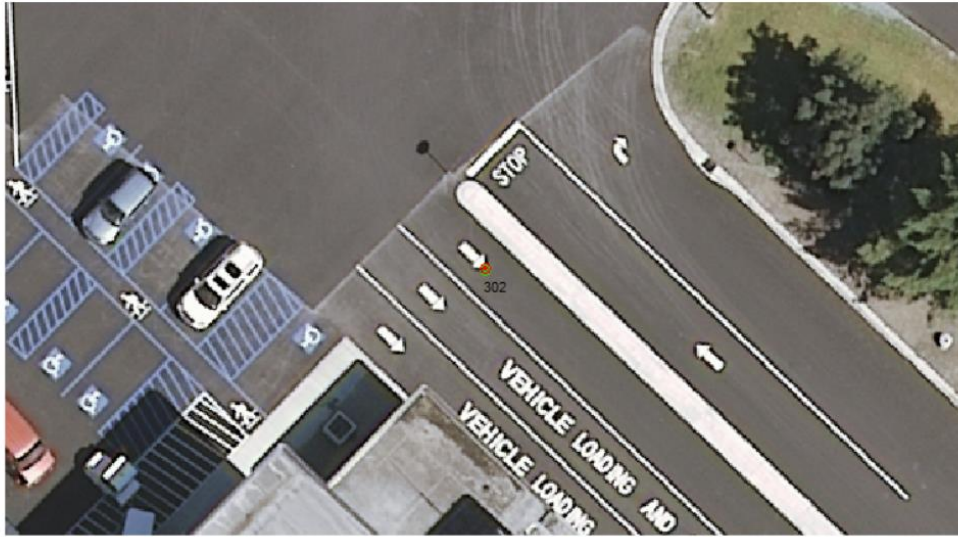
Figure 11: Image displaying the co-registration of a GPS ground check point and the rectified imagery in the Ketchikan site.
