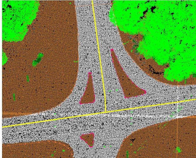
Figure 12. Completed classifications with road islands retained in Class 2 Ground and road surfaces in Class 13
