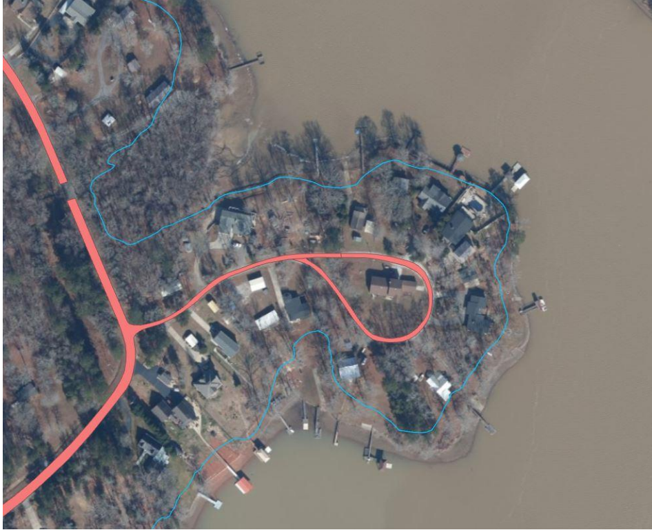
Figure 15: Flooding in the lake resulted in the hydro breakline being inset significantly along the shoreline
