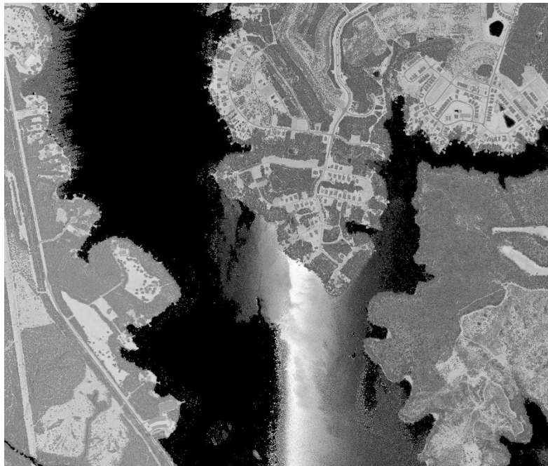
Figure 6. Intensity example showing high reflectance values over water
