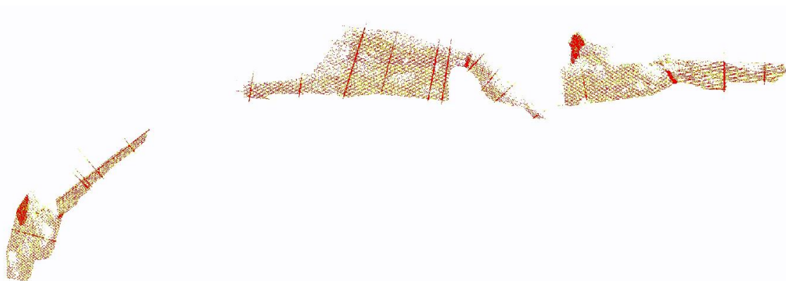
Figure 5. Interswath raster generated using proprietary software and symbolized according to the ranges specified above. Inter-swath relative accuracy passes specifications.
