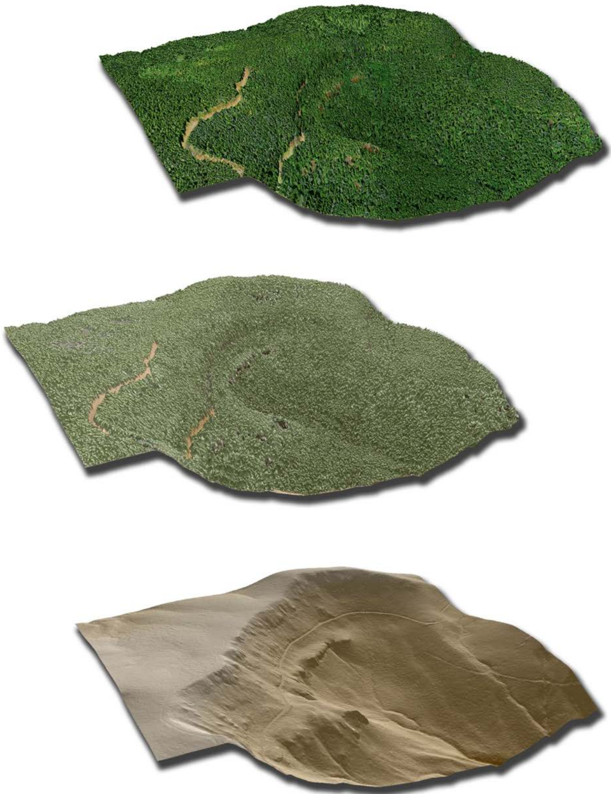
Figure 5.7. Forested area 6 miles south of Grand Ronde. Top: LiDAR derived highest hit face colored by 2009 NAIP imagery. Middle: LiDAR derived highest hit surface colored by vegetation height. Bottom: LiDAR bare earth surface colored by elevation.
