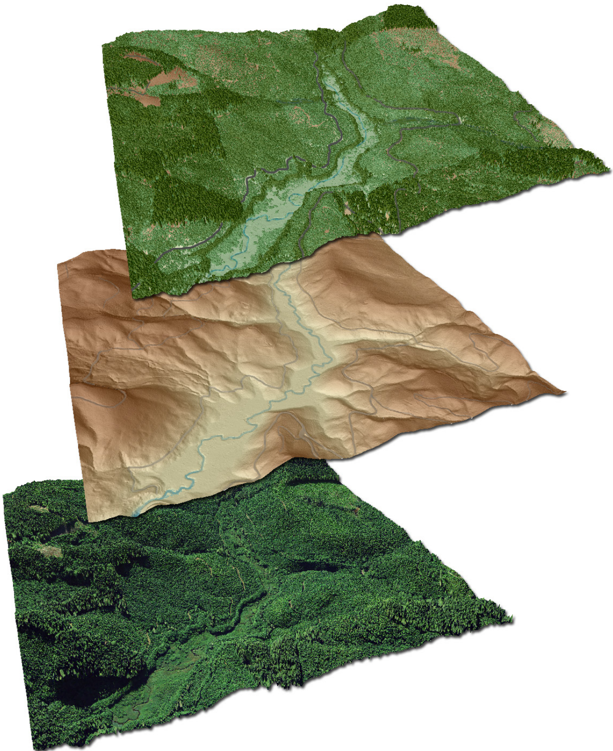
Figure 5.1. View of Nestucca River, one mile north east of McGuire Reservoir. First image derived from highest hit LiDAR, second image derived from bare earth LiDAR, third image derived from NAIP orthophoto draped over highest hit LiDAR.
