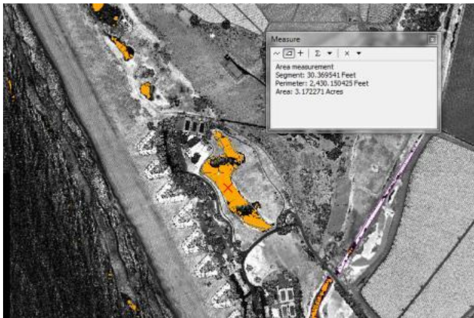
Figure 13 - Tiles C64045_40815 and C6045_40800. Full point cloud shows a water body larger than 2 acres that has not been captured
