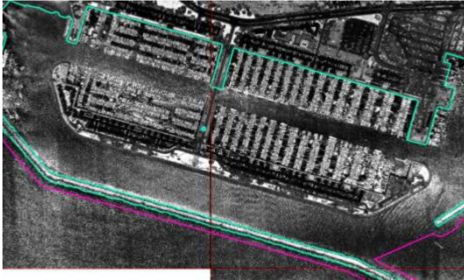
Figure 14 - Tile C4350_37020. Full point cloud intensity shows an “island” in the tidal water. This feature should be collected in the breaklines.
