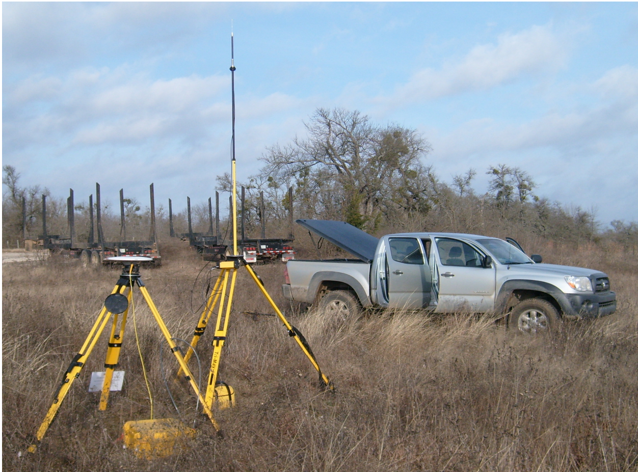
Trimble GPS survey equipment configured for collecting RTK data.
