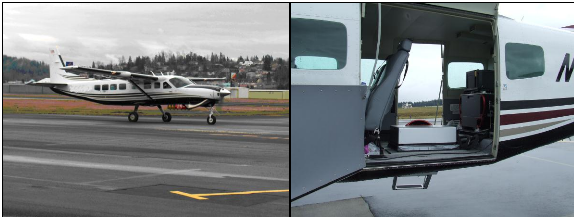
The Cessna Caravan is a powerful, stable platform, which is ideal for the often remote and mountainous terrain found in the Pacific Northwest. The Leica ALS60 sensor head installed in the Caravan is shown on the right.
