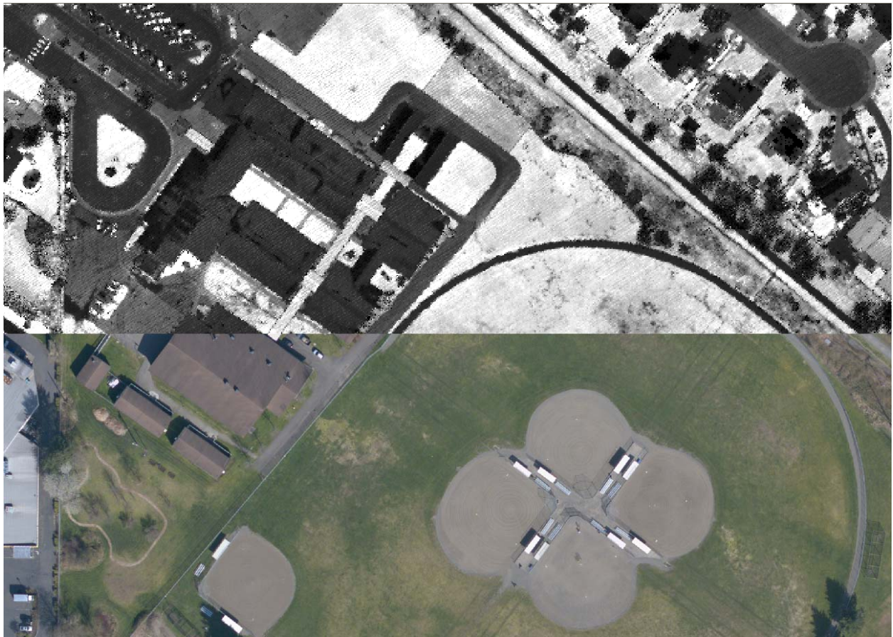
Figure 3. Example of co-registration of color images with LiDAR intensity images
