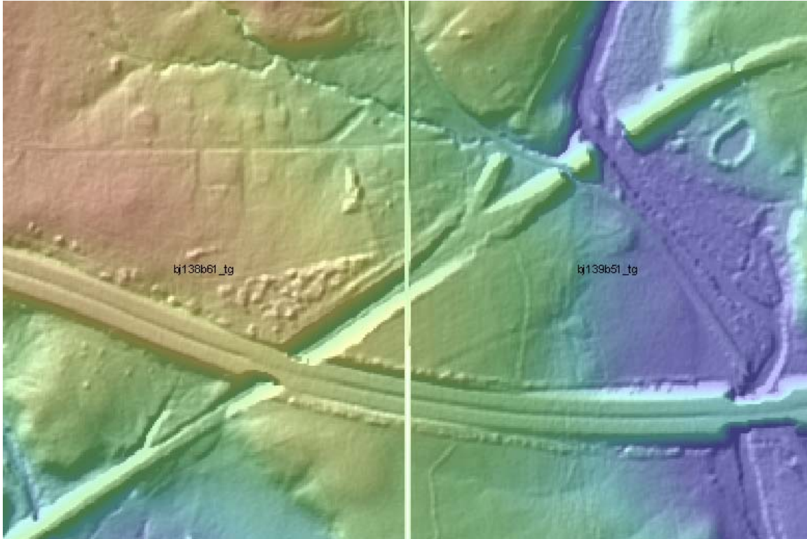
Figure 8 - TIN Grid and Hillshade illustrating inconsistent bridge editing (BJ138b61).
