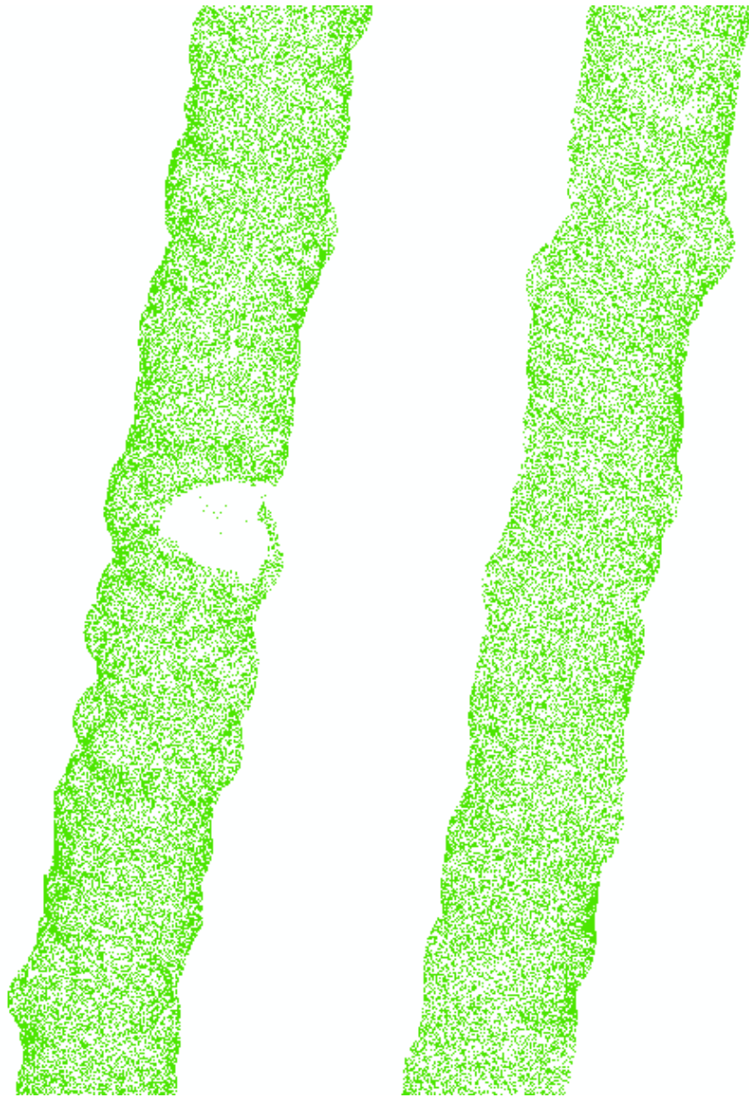
Figure 4–Intra-swath relative accuracy. This image shows a portion of the dataset; areas where the maximum difference is \leq 6 cm per pixel within each swath are colored green. This open flat area is acceptable for repeatability testing. Intra-swath relative accuracy passes specifications.
