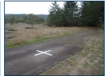
Above: Example of co-registration of color images with LiDAR intensity images. Below: Examples of permanent air targets located within the OLC Big Windy project area.
