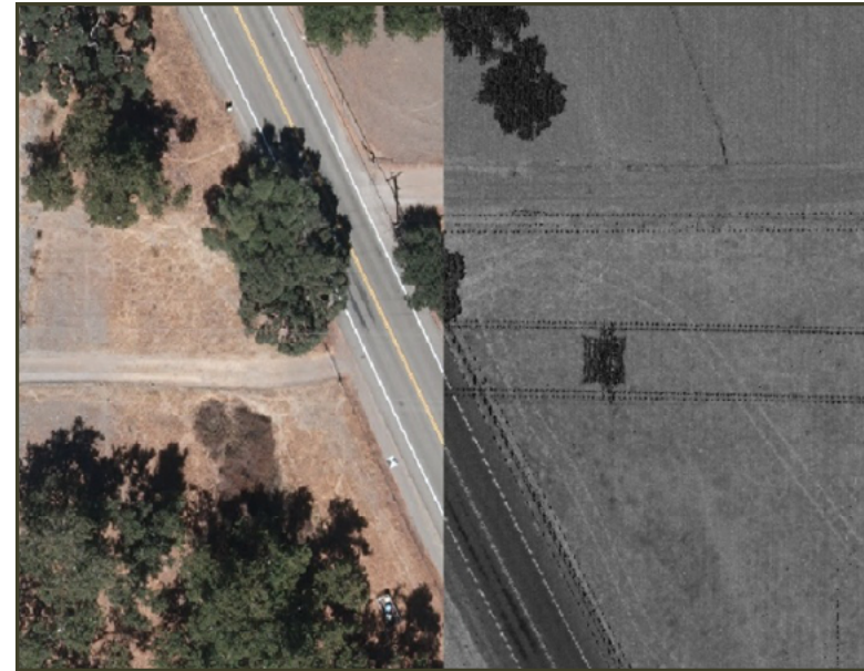
Above: Example of co-registration of color images with LiDAR intensity images. Below: Examples of permanent air targets located within the OLC Big Windy project area.
