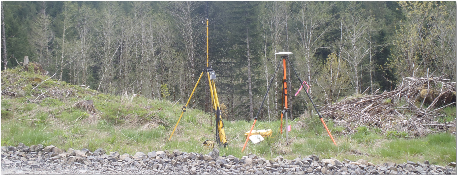
Base station and radio unit set up over control "CLACK_10"
