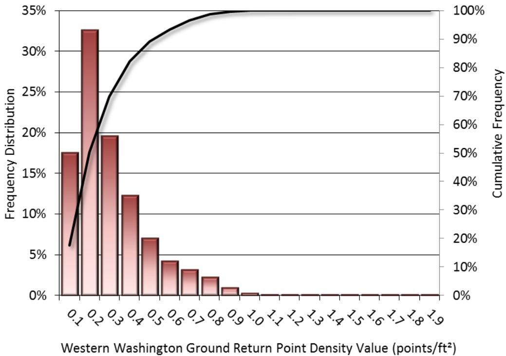
Figure 7: Frequency distribution of ground-classified return point density values per 300 x 300 ft cell
