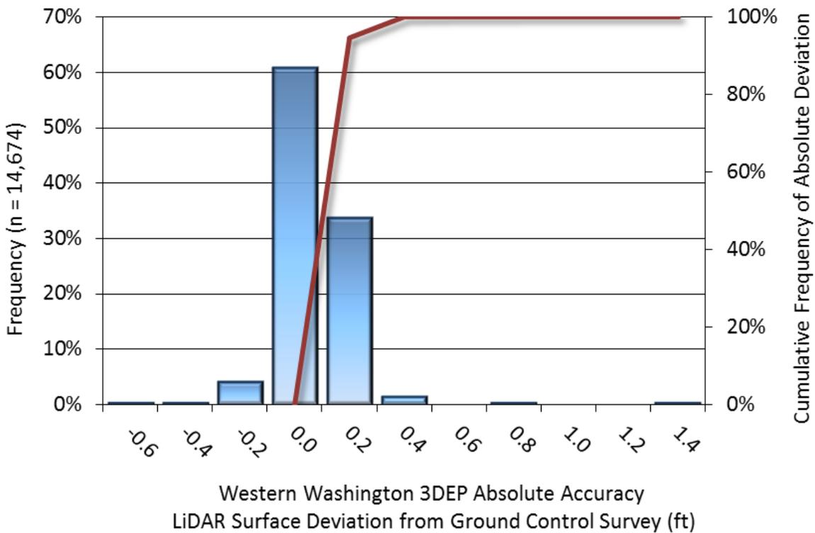
Figure 10: Frequency histogram for LiDAR surface deviation from ground control point values
