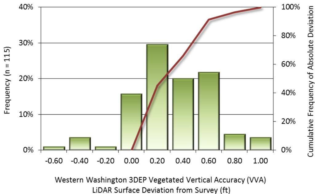
**Figure 11: Frequency histogram for LiDAR surface deviation from all land cover class point values (VVA)**
