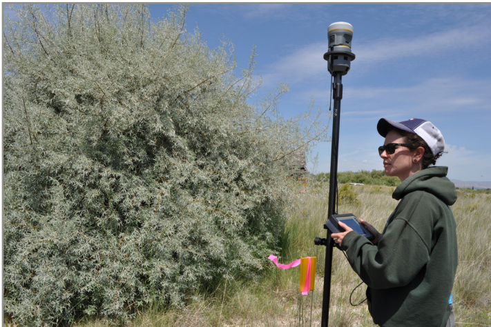
Field surveyor collecting land class RTK points.
