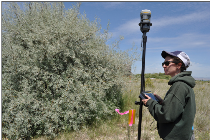
Field surveyor collecting land class RTK points.
