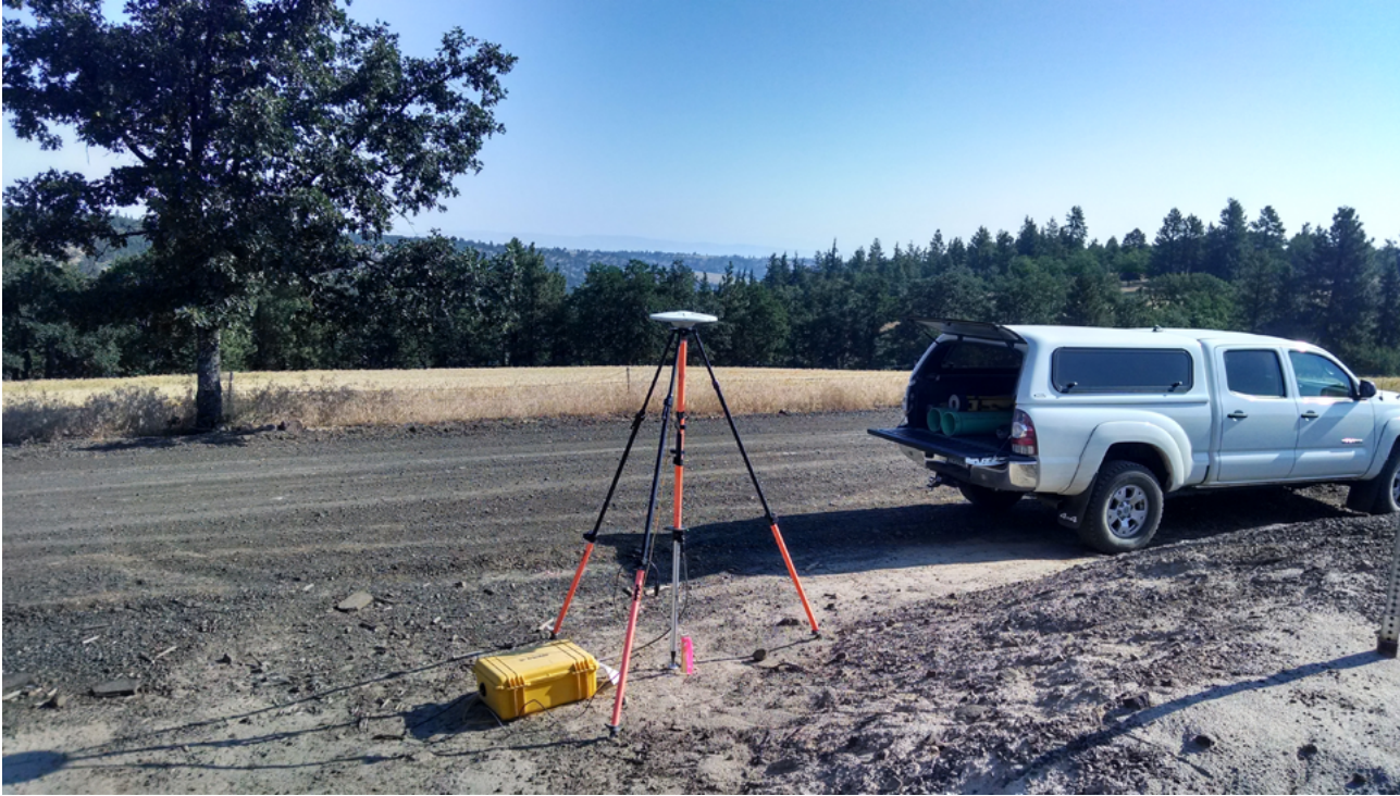
Trimble R7 Receiver set up over GPS monument WASCO_02.
