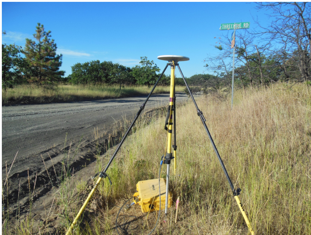
Trimble R7 Receiver set up over GPS monument WASCO_03.
