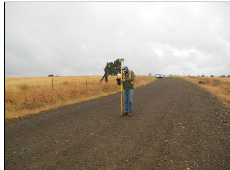
WSI ground professional collecting ground survey points in OLC Wasco County study area.
