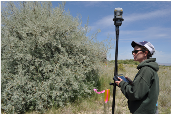
Field surveyor collecting land class RTK points.
