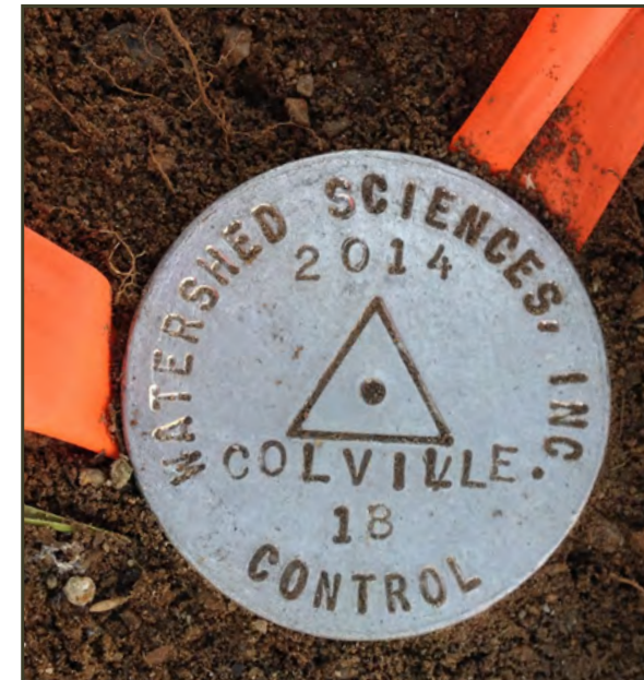
Below: Survey monument COLVILLE_18
