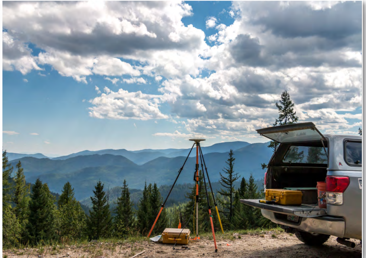
Base station set up over a survey monument within the Colville study area.
