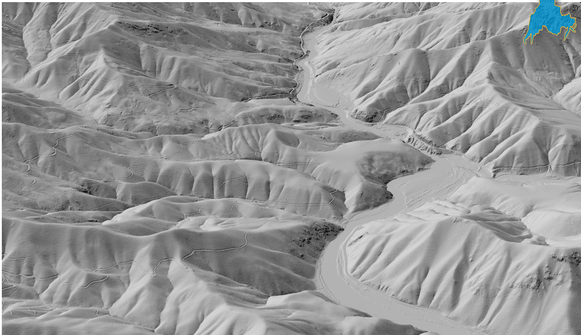
Hillshade of LiDAR-derived 1m DEM. Carpenters Island on the Rogue River, Oregon. View to the East.
