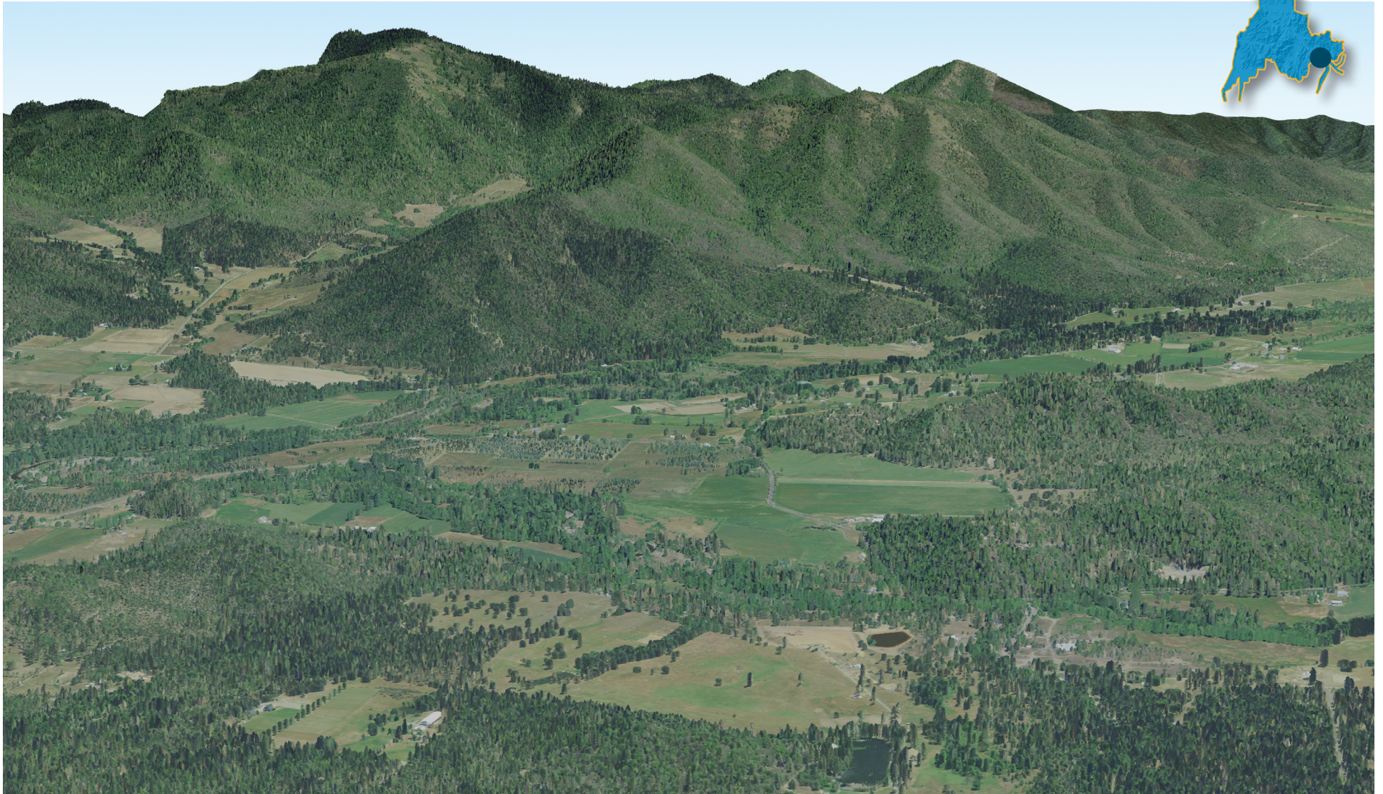
LiDAR point cloud with RGB extraction from 2009 NAIP imagery. Forested hills north of Applegate, Oregon. View to the East.
