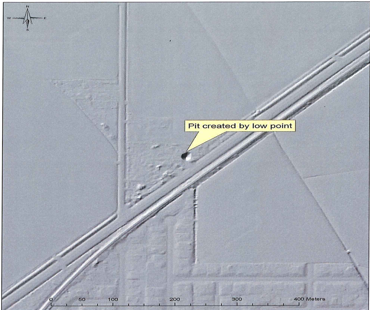
Figure 8. Example of “Pit” caused by low point in ground model. Pits are caused when standing water absorbs the lidar pulse. Pits are evident in ground model as the lowest point elevation is assigned to the grid cell value. Inversely the pit is not observable in the highest hit model as the highest point elevation is assigned to the grid value.
