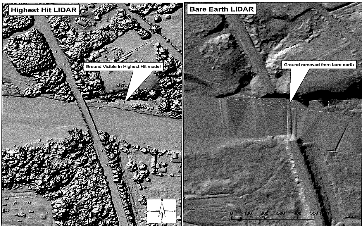
Figure 6. Example of missing ground in lidar bare earth data. Ground is clearly visible in highest hit model, but has been removed from the bare earth model. This type of classification error is common near water body features
