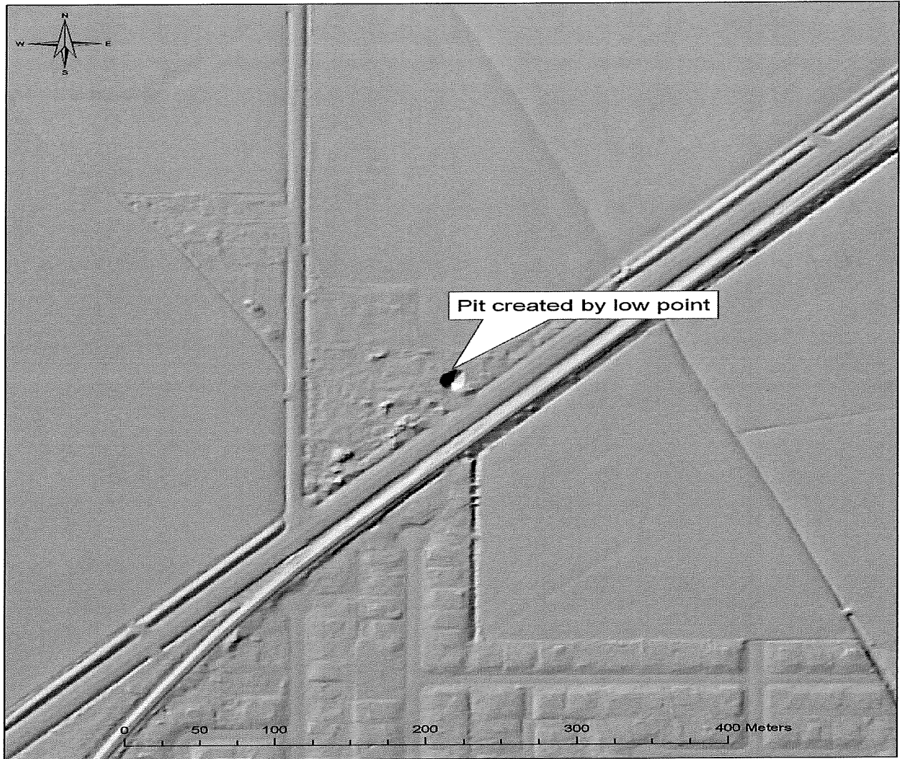
Figure 8. Example of “Pit” caused by low point in ground model. Pits are caused when standing water absorbs the lidar pulse. Pits are evident in ground model as the lowest point elevation is assigned to the grid cell value. Inversely the pit is not observable in the highest hit model as the highest point elevation is assigned to the grid value.
