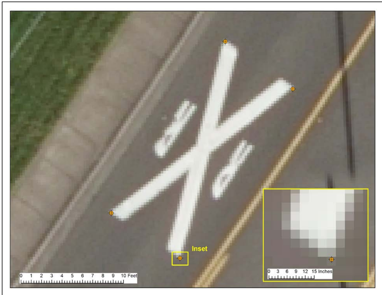
Figure 8. Aerial Target feature used to orthorectify imagery.
