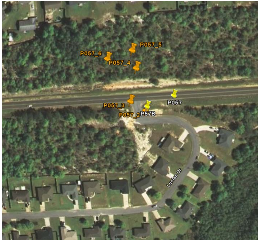
Figure 3. Example “Site” with Yellow Markers (NGS Benchmark and TBM) as Control and Orange Markers as GCPs
