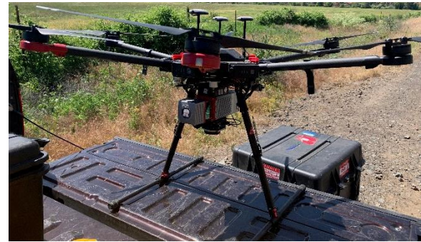
Riegl MiniVUX-1UAV LiDAR sensor mounted on a DJI Matrice 600.
