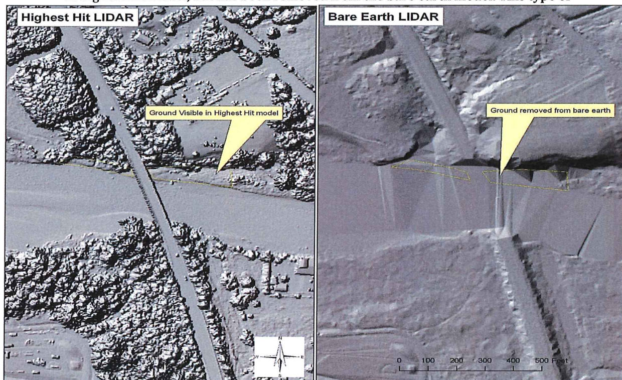
Figure 6: Example of missing ground in lidar bare earth data. Ground is clearly visible in highest hit model, but has been removed from the bare earth model. This type of
