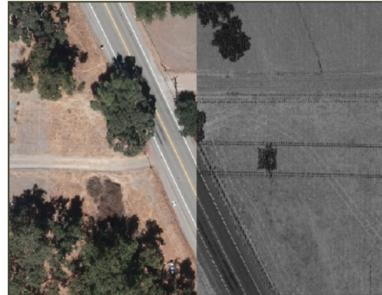
Above: Example of co-registration of color images with LiDAR intensity images. Below: Examples of permanent air targets located within Lane County project area.
