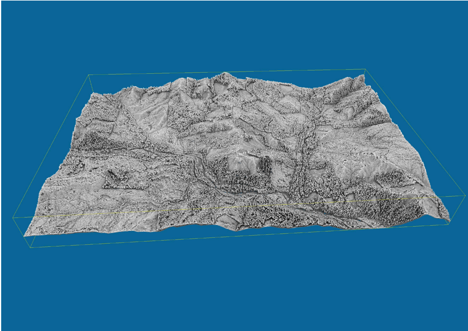
Highest Hit DEM of section of Delivery Area Two.
