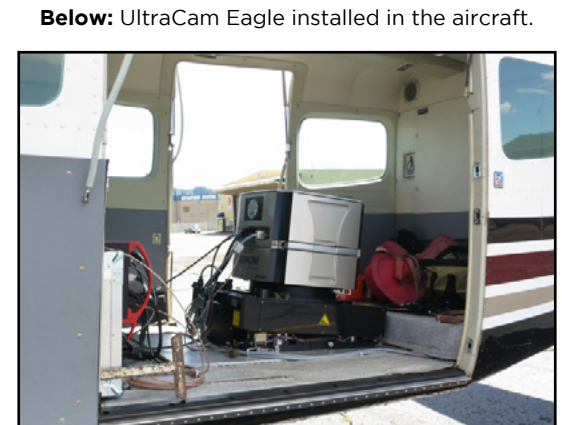
Below: UltraCam Eagle installed in the aircraft.
