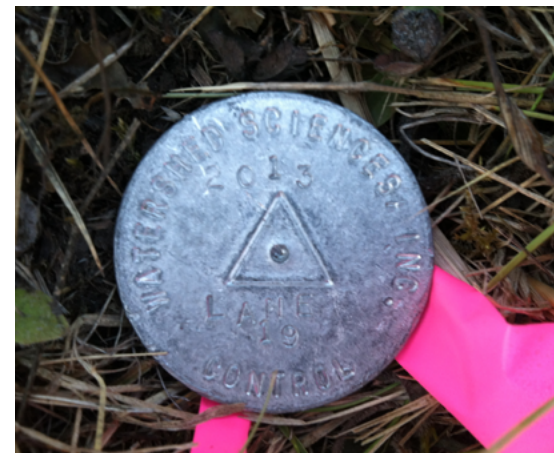
"Lane 17" and "Lane 19" survey caps.
