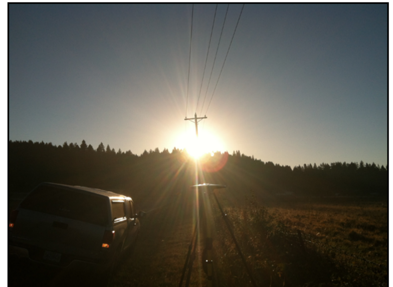
Below: Trimble R7 set up over Lane_19.
