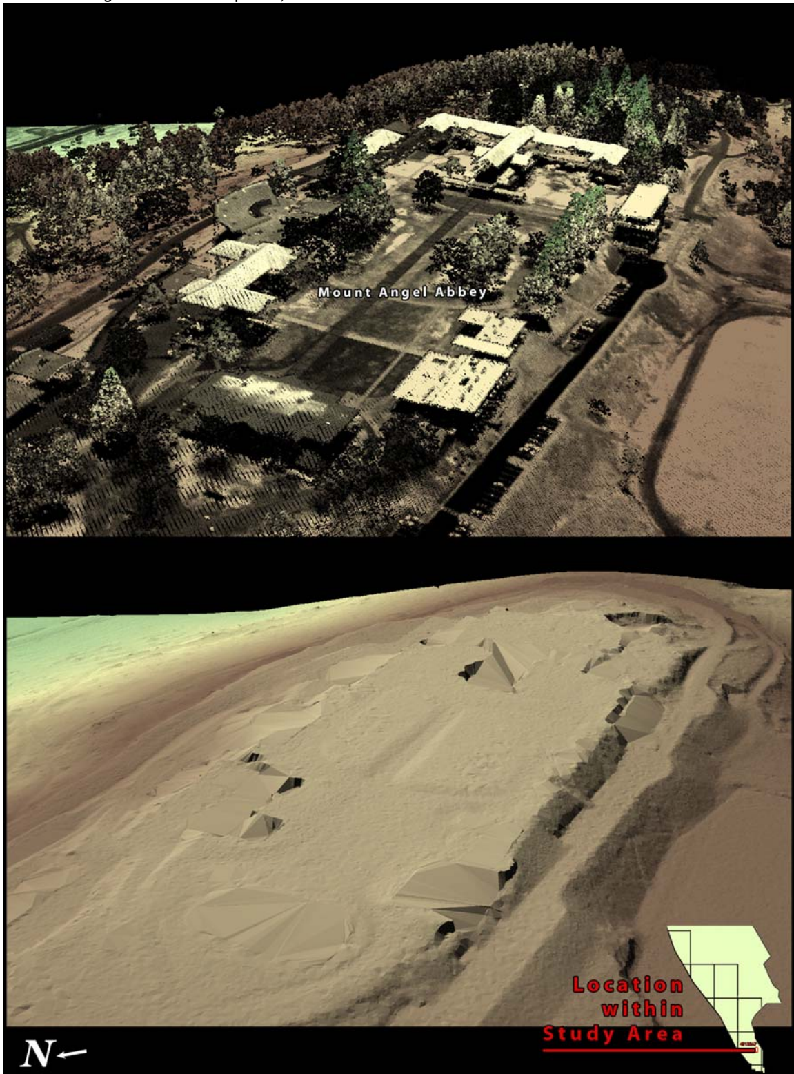
Figure 27. 3-d oblique view of LiDAR-derived surfaces in 0.75' Quad 45122A7223-224,403-404, showing the Mount Angel Abbey in the DOGAMI study area (top image derived from all points, bottom image derived from ground-classified points).
