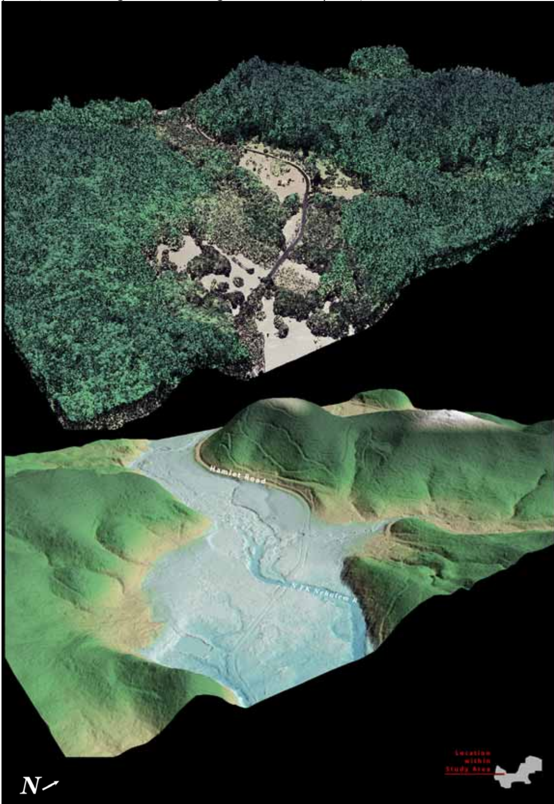
Figure 24. 3-d oblique view of LiDAR-derived surfaces in Quad 45123G6115, showing the North Fork Nehalem River and Hamlet Road in the ODF North Study Area (top image derived from all points, bottom image derived from ground-classified points).
