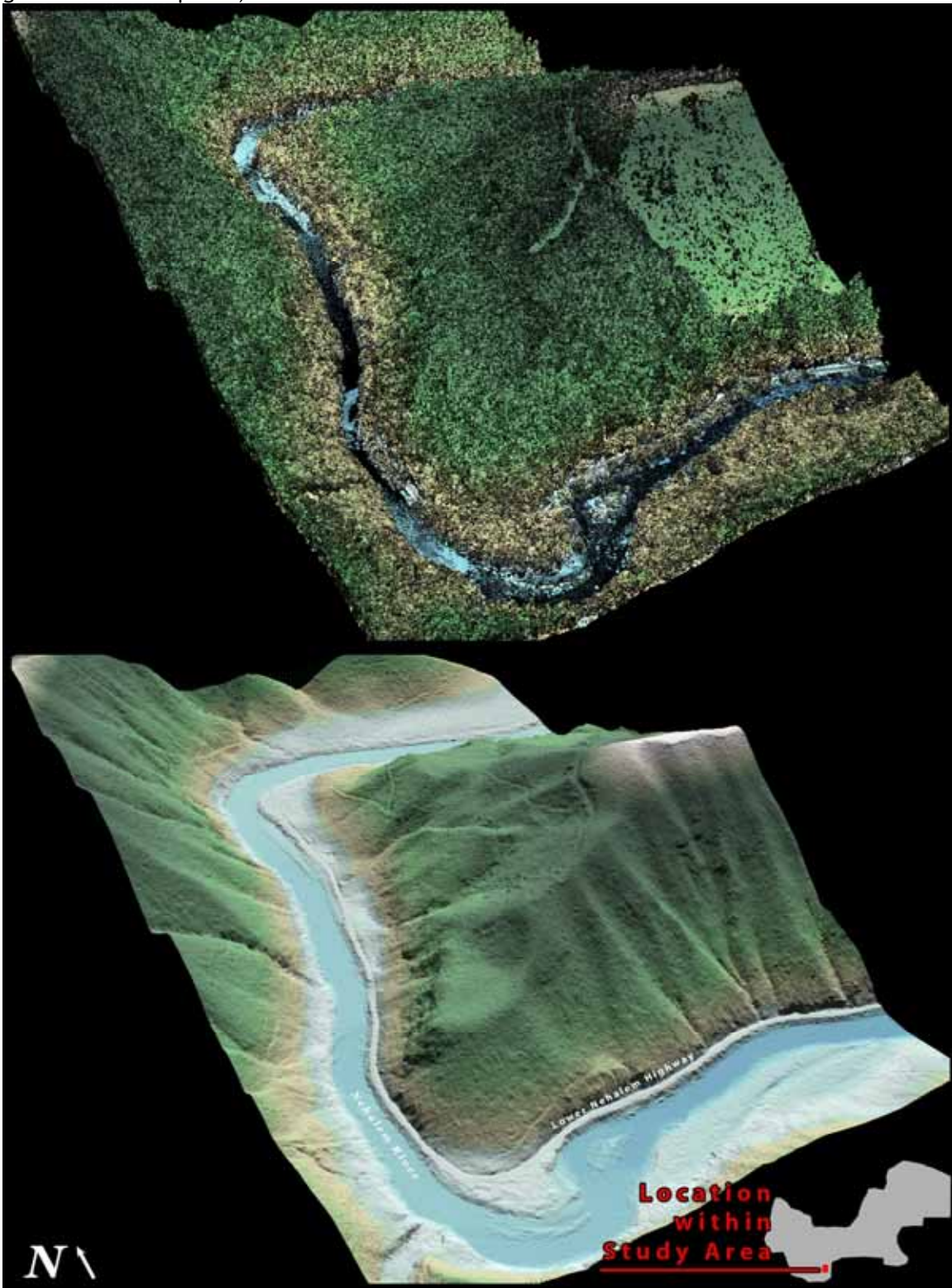
Figure 25. 3-d oblique view of LiDAR-derived surfaces in Quad 45123G6414, showing the Nehalem River and the Lower Nehalem Highway, just inside the Clatsop State Forest boundary in the ODF North Study Area. (Top image derived from all points, bottom image derived from ground-classified points).
