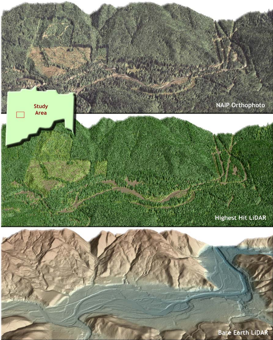
Figure 39. 3-d oblique view of LiDAR-derived surfaces looking south over the Wilson River near the North Fork confluence.
