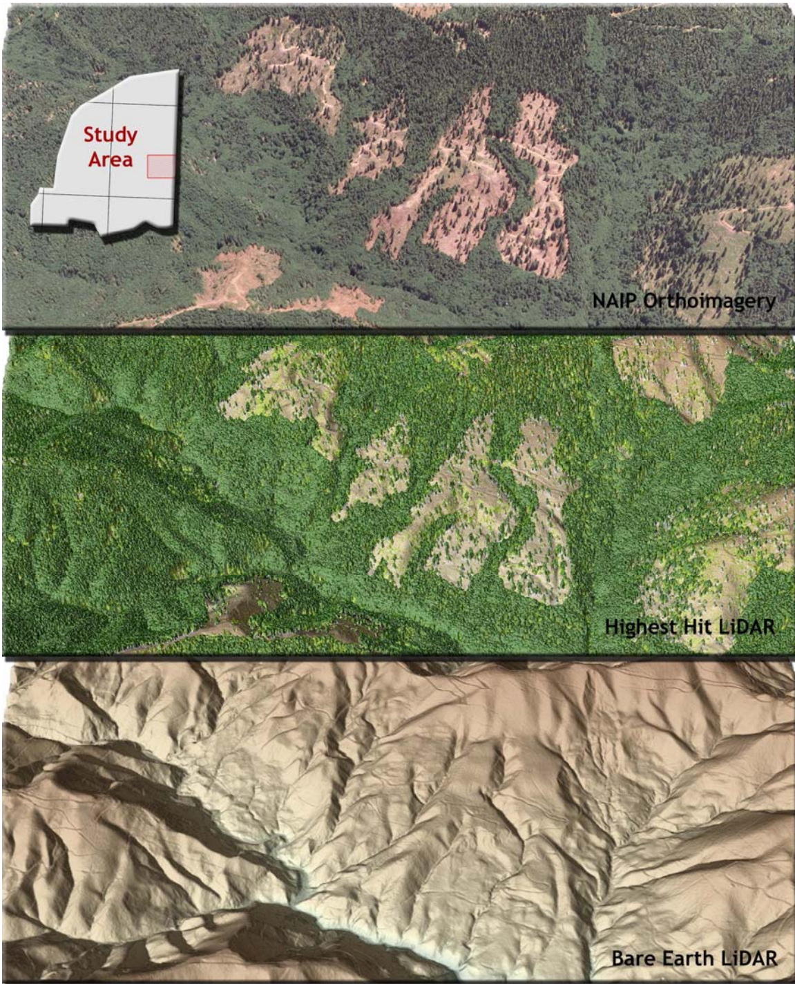
Figure 37. 3-d oblique view of LiDAR-derived surfaces in 7.5' Quad 45123E6, showing the upper portion of the Little North Fork Wilson River watershed in the ODF South study area.
