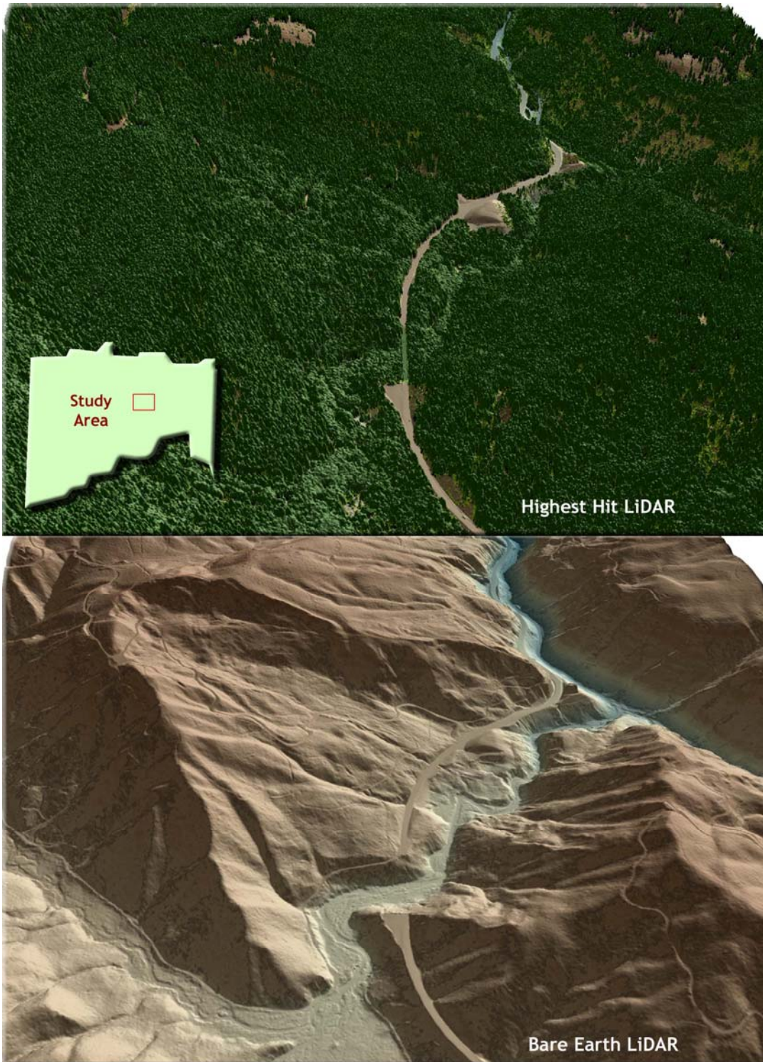
Figure 6.15. 3-d oblique view of LiDAR-derived surfaces showing an historic landslide along Devils Lake Fork, between Elliot Creek and Drift Creek.
