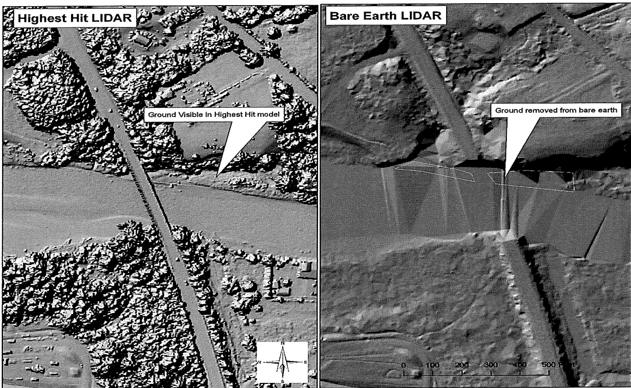
Figure 6. Example of missing ground in lidar bare earth data. Ground is clearly visible in highest hit model, but has been removed from the bare earth model. This type of classification error is common near water body features
