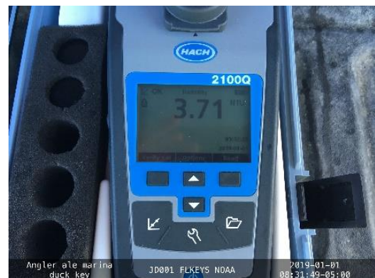
Figure 3: Hach Turbidity Meter
