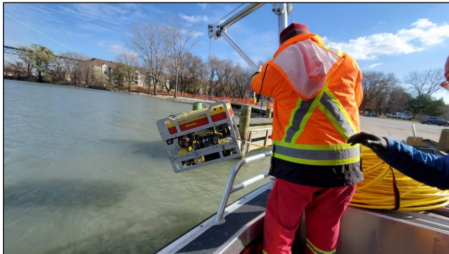
Figure 8: Launching the Falcon ROV with the ULS off the side of the vessel.
