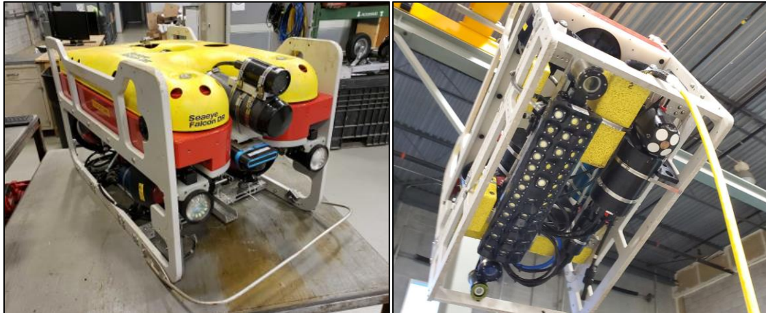
Figure 4: Seaeye Falcon DR ROV (left) and underside equipped with ULS-500 and INS (right)
