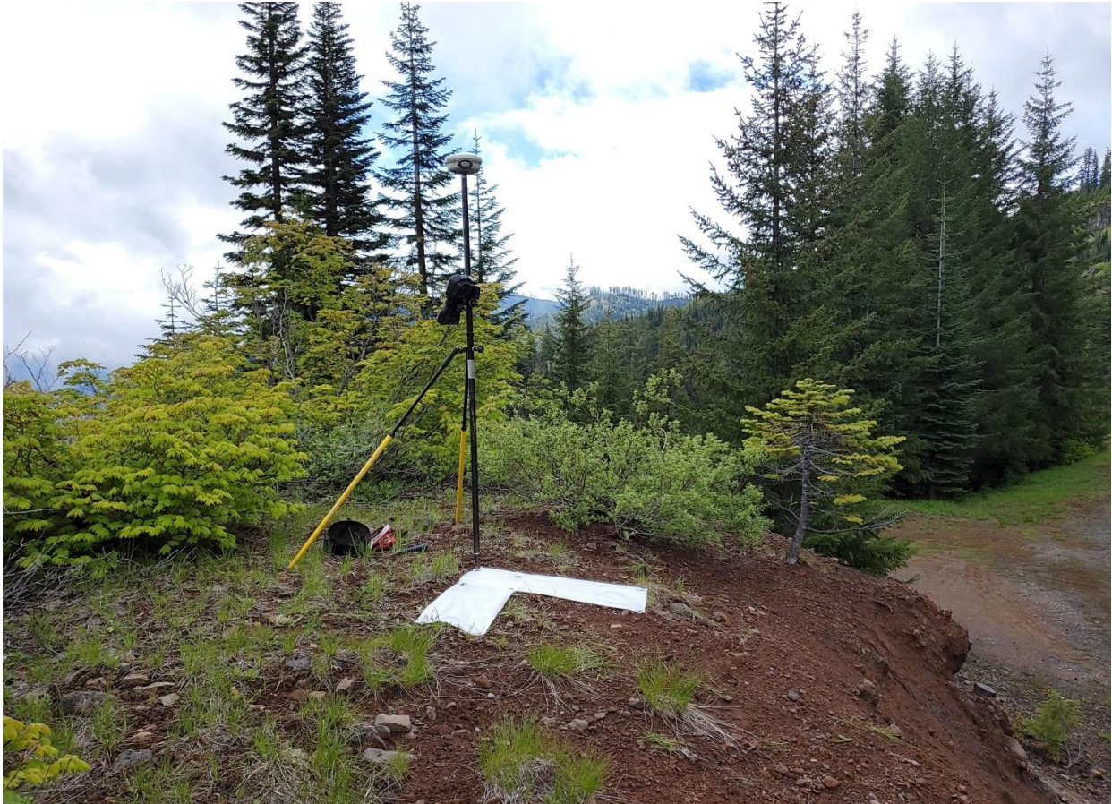
Aerial Target acquisition equipment set up in the Blue Pool Lidar & Imagery project area.
