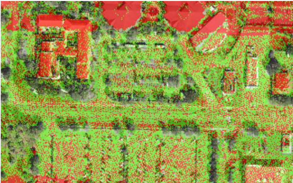
Figure 6. Intraswath DZ raster for the Tampa Bay South TopoBathymetric Lidar, Imagery, and Shoreline Mapping Project. This image depicts a spatial subset of the dataset; flat, open areas are predominantly shaded green as they are within 6 cm whereas sloped and/or vegetated terrain is shaded red, as data in these locations exceeds 6 cm maximum difference. Buildings and spurious “only returns” (i.e., noise) also appear as red pixels.
