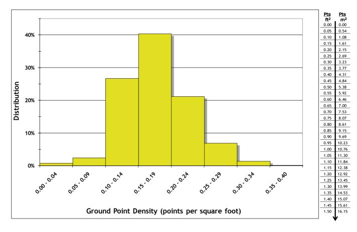
**Figure 4.4.** Ground-classified laser point density per 0.75' USGS Quad for data delivered to date.
