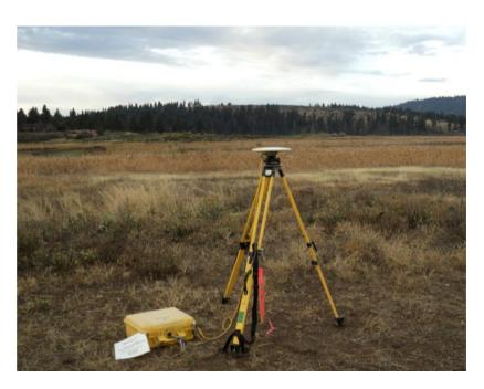
Indexed by time, these GPS data records are used to correct the continuous onboard measurements of aircraft position recorded throughout the mission. Control monuments were located within 13 nautical miles of the survey area(s).
