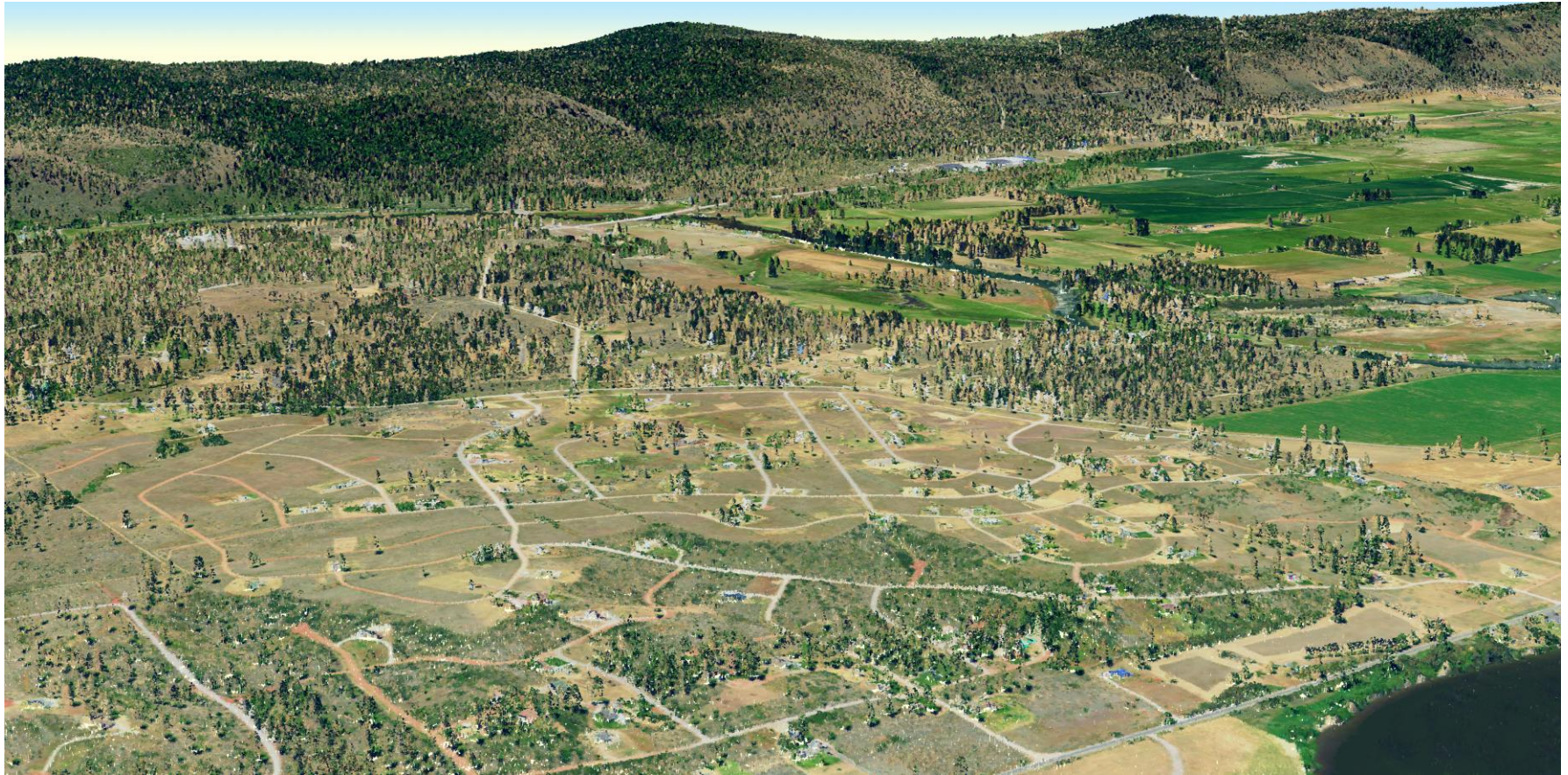
Figure 5.6. Residential development located one1 mile west of Highway 97 and Highway 62 intersection, four miles south of Chiloquin, OR. View looking East. Image is a three dimensional LiDAR point cloud with RGB values extracted from a 2009 NAIP orthophoto.
