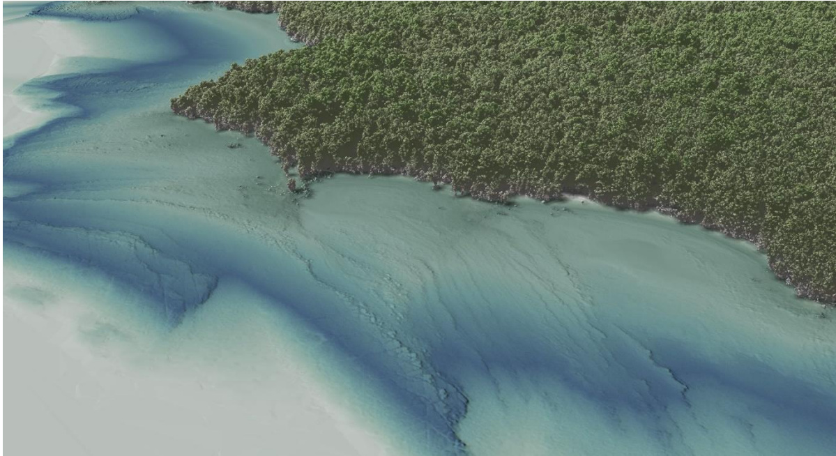
Figure 20: View looking southeast over Lake Champlain in the NOAA Finger Lakes AOI. The image was created from the lidar bare earth model overlaid with the above-ground point cloud and imagery and was colored by elevation.
