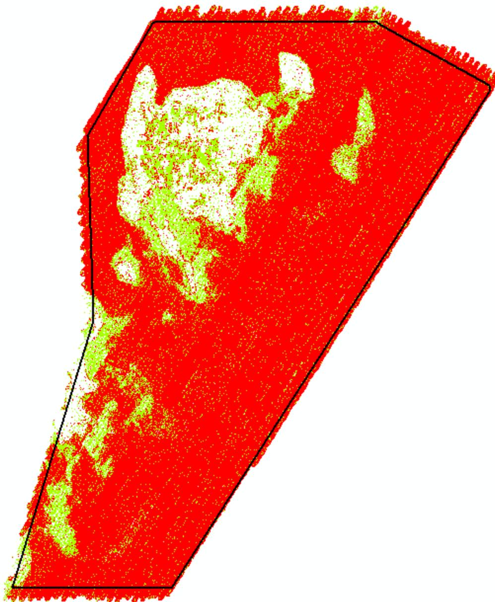
**Figure 6. Intraswath rasters for the Green Bay Topobathy Project. Flat, open areas are colored green as they are within 6 cm whereas sloped terrain is colored red because it exceeds 6 cm maximum difference, as expected, due to actual slope/terrain change, water surface, and/or vegetation.**
