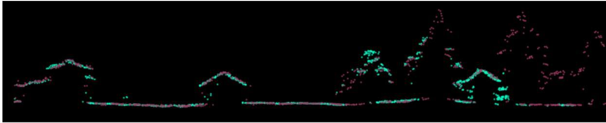
Figure 7. Two separate flight lines are differentiated by color (teal/maroon) to determine whether horizontal misalignments are present. This is a representative example; there is no visible offset between these flight lines.
